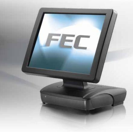
Glaive Pro is fan-less POS terminal featuring an Intel® Atom™ 1.6 GHz processor and N270 chipset, providing strong graphic performance. The fan-less design prevents any inhalation and accumulation of dust particles, increasing the longevity of the terminal.
